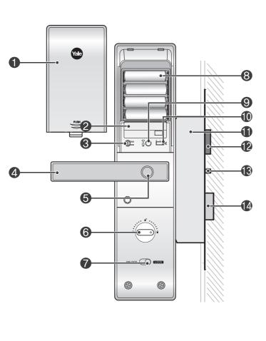
4. Main Body (Main Body, installation on the inside of the door)
