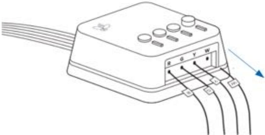
4. Remove the PEK wires attached to the control board. This can be done while simultaneously connecting the wires from the CWA to the control board.
