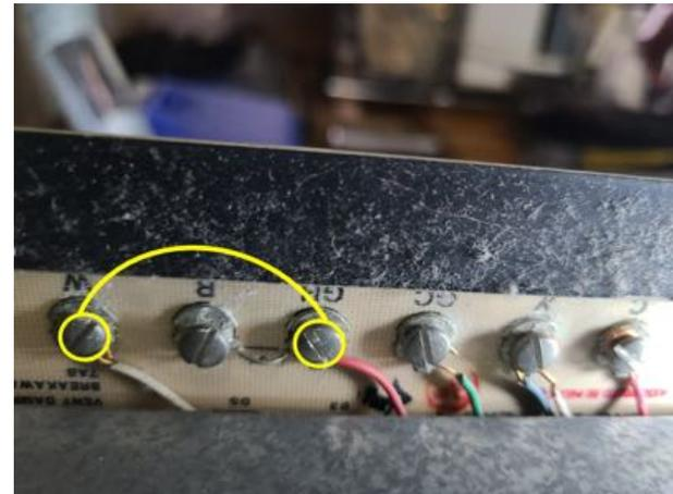
1. Disconnect the wire connected to GH and connect it to R.
