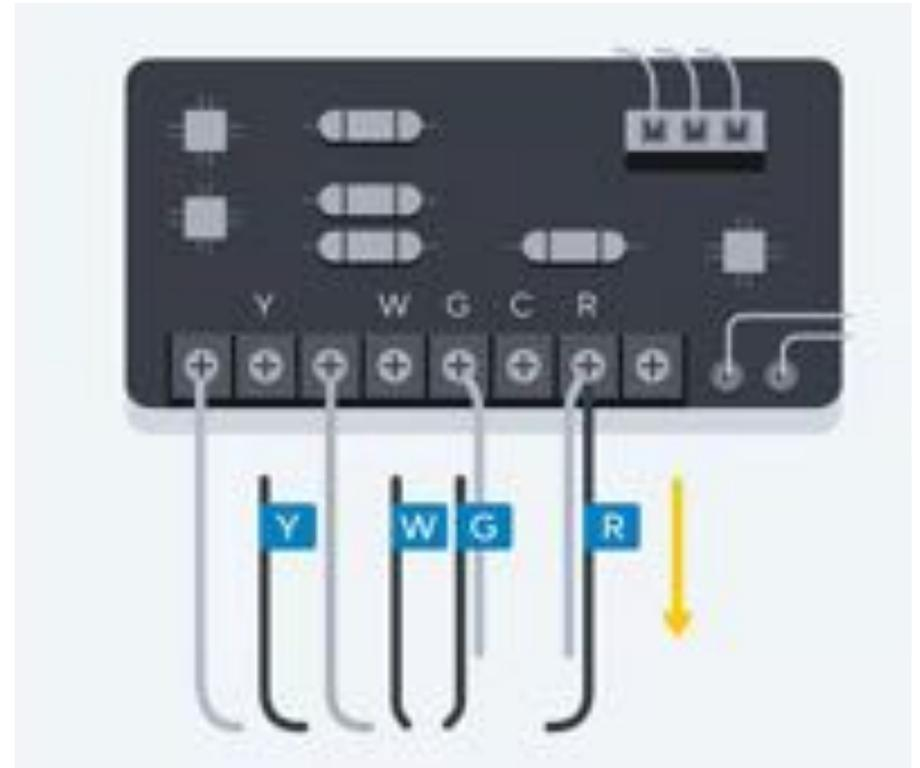
**Step 7. Connect the labeled wires from the control board to the CWA**
