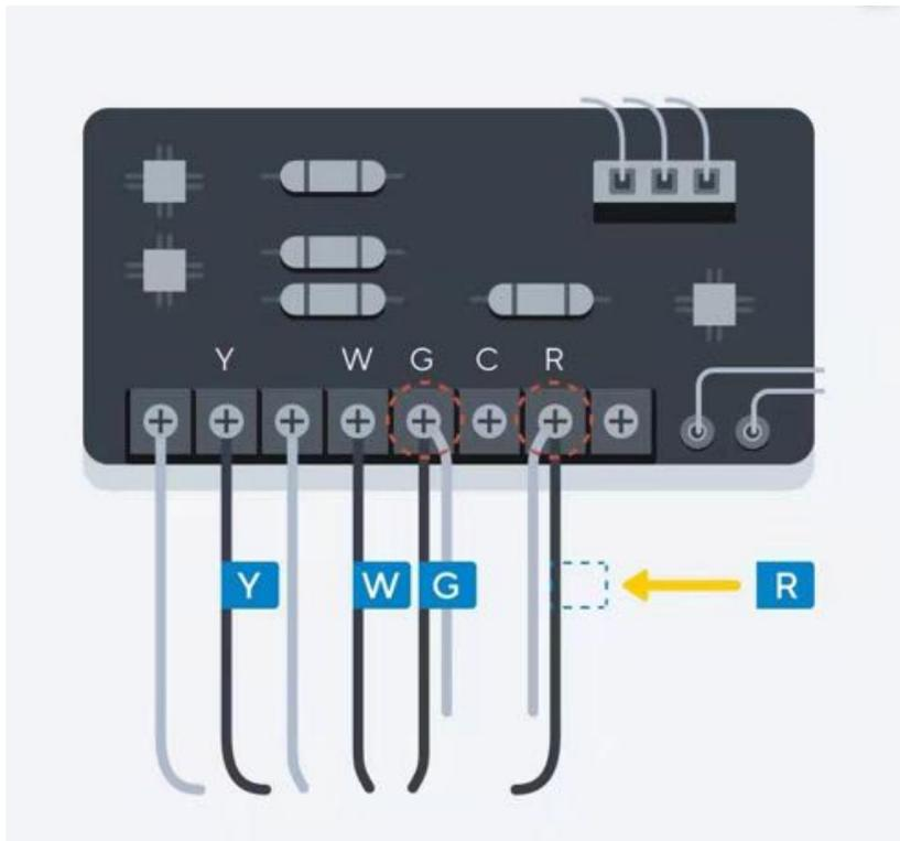
**Step 6. Disconnect the labeled wires from the control board**
