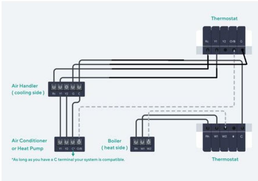
With dual transformer setups, you will have two R wires—one from the cooling transformer (RC) and one from the heating transformer (RH).
