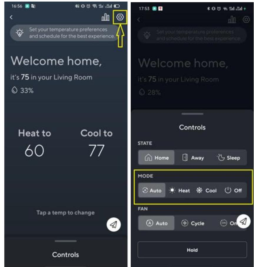
To enable this system mode, tap on **Controls** on the Main Menu to display the control options and then select **Auto** under modes to activate it.
