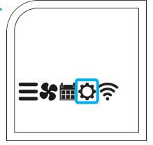
This icon opens the installation settings menu. In this menu, you can adjust advanced preferences for special applications. Select the gear icon, then after IS appears on the screen, select yes to begin the installation settings flow. For more information about the installation settings, please view the "Installation Settings Guide".
