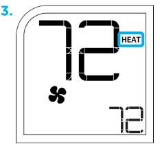
The selected system mode (either HEAT, COOL, AUTO, or OFF) is shown to the right of the ambient room temperature.
