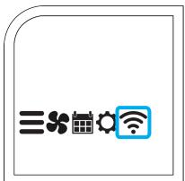
This icon opens the WiFi connection menu. In this menu, you can choose to connect or disconnect to a WiFi network, or temporarily turn-off your WiFi connection. Select "set" to establish a new network connection. Select "off" to temporarily disable the connection. Lastly, select "on" to reconnect to your WiFi network. For more information about connecting to the network, please view KONO's "Installation Manual".
