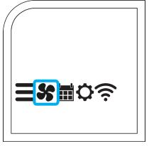
This icon opens the fan mode menu. In this menu, you can set your fan to AUTO, ON, or IAQ. Auto will run your fan when your system is actively heating or cooling. ON will run your fan continuously. Lastly, IAQ will periodically run your fan so that fresh air is cycled through your home even when your system isn't heating or cooling. If you set a filter life value in the installation settings, you'll be able to check the remaining life of your filter in the fan settings menu.
