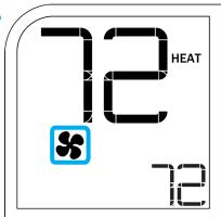
The active fan status is shown by the icon below the ambient room temperature. If it is off, your fan is not running. If it is on, your fan is running. Please note that your fan will run depending on your selected fan mode (either AUTO, ON, or IAQ).
