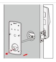
**2:** Align and secure mounting plate with adhesive strips. Guide connection cables through the hole and secure to the lower left notched hole.
