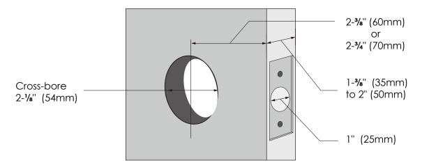
Deadbolt slot must align to the center of the door hole. Adjust as shown if needed.
