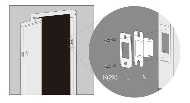
**IMPORTANT:** because doors and frames vary in design it may be necessary to make slight adjustments to your strike plate and/or dust box in order to ensure smooth deadbolt operation. **This is very important.** If the deadbolt is binding or catching in any way the lock will sound an alarm (rapid beeping) indicating it cannot close due to misalignment and/or excessive rubbing or binding.
