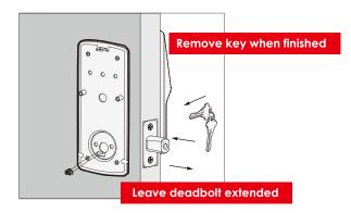
4: Use the key to ensure deadbolt locks and unlocks smoothly (no binding or rubbing). IMPORTANT: when finished, leave the deadbolt extended and remove the key before proceeding to the next step.
