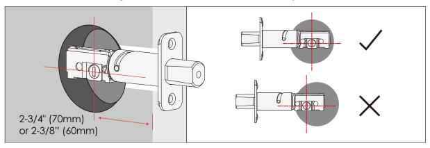
The deadbolt comes set to 2-3/4" (70mm). Adjust length to 2-3/8" (60mm) if necessary. (wear gloves to protect from possible pinching).
