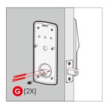
**3:** Insert and tighten by hand 2 **G** screws located on the left and right of the blade. Check alignment and tighten with screwdriver until mounting plate is securely placed on door.
