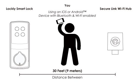
**TIP:** The Secure Link requires a strong wireless signal for optimal performance. Make sure the Secure Link will be installed in a location with a strong 2.4 Ghz wireless signal. Sometimes distances between Wi-Fi hub and lock can vary due to circumstances. If you are having difficulty setting up optimal range of 30/ft or less, we're here to help. Call our customer care team: (669) 500 8835, or visit Lockly.com/help for suggestions and troubleshooting tips.
