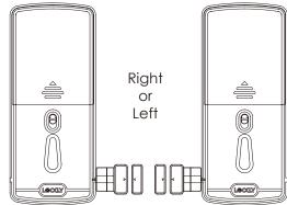
The interior assembly comes with the pre-installed wired door sensor setup for a right swing doors with 2 ¾" (70mm) backset\*.
