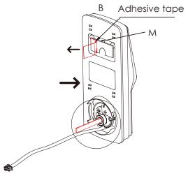
Peel film from adhesive strips and make sure torque blade is in the vertical position with the deadbolt extended. Place assembly and torque blade through the deadbolt slot and guide connection cables through the cross-bore hole under the deadbolt as shown. Complete mounting by aligning and securing until flush to exterior door surface.
