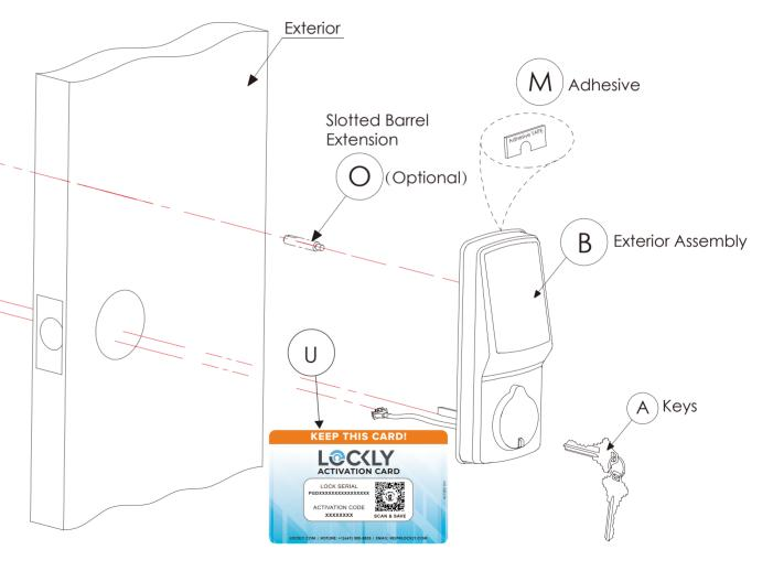
Lockly Secure Pro can be fitted for both right swing doors and left swing doors.
