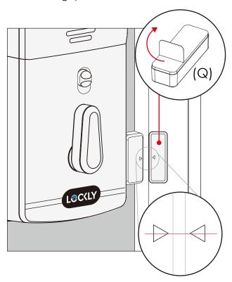
**NOTE:** When properly installed, the Lockly logo blinks red when door opens and closes.
