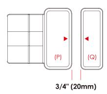
The sensors need to be as close to level as possible. If needed, use the adhesive foam pad(s) to adjust the height of the wired sensor.
