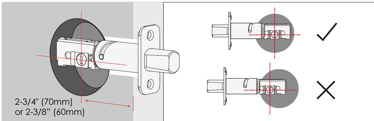
The deadbolt comes set to 2-3/4" (70mm). Adjust length to 2-3/8" (60mm) if necessary. (wear gloves to protect from possible pinching).
