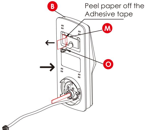
\*This hole (O) is for the optional Slotted Barrel Extension provided for stabilizing your lock. It will require drilling extra hole on your door (See template as provided). Alternatively, you may use the double-sided adhesive tape provided which serves the same purpose if you do not want to drill a hole. If you drilled a hole, securely tighten the post with a flathead screwdriver by turning it clockwise before mounting on your door.
