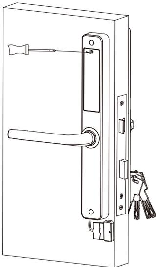
2. Check the lock functions according to user manual after installing the batteries. Use the battery cover to secure the battery compartment and fasten with screw.
